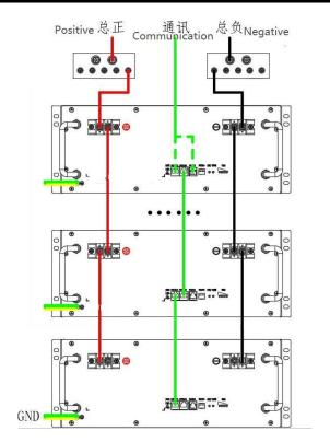
Figure 15-1 Parallel connection diagram of battery box
